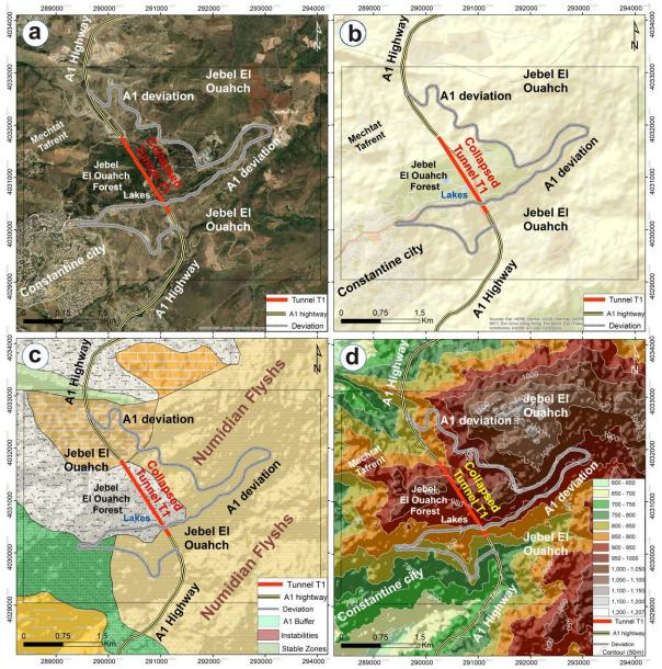
Figure 2. (a) The new Djebel El-Ouahch deviation on satellite images. (b) The new Djebel El-Ouahch deviation on street map. (c) The new Djebel El-Ouahch deviation on numidian (beige) formations.(d) The new Djebel El-Ouahch deviation on steep landscape (DEM).
