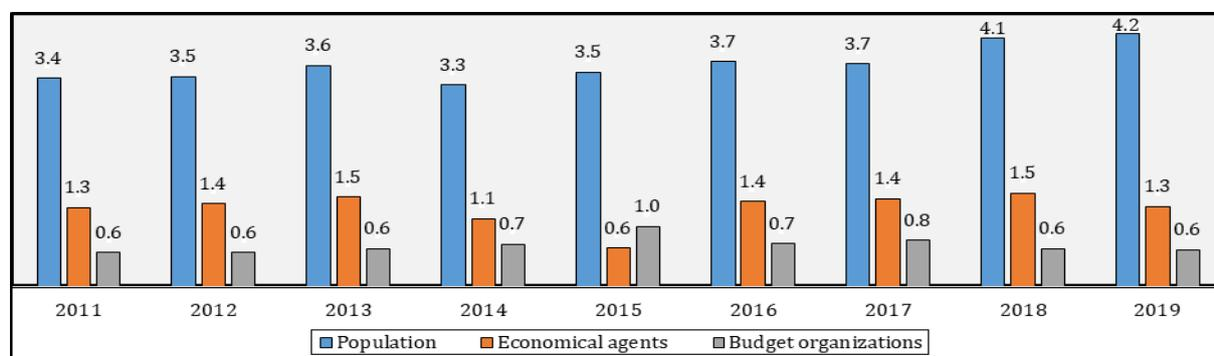
**Figure 17.** Dynamics of the volume of wastewater discharged in the public sewerage systems from RD Nord by categories of users, mil. m<sup>3</sup>.
